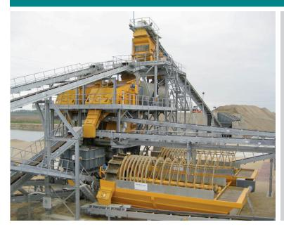
Combination of screening machines and wet processing machines (log washer, sand trap) for cost efficient production of high-grade aggregates
